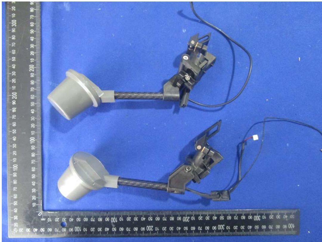
RTK Antenna Location
