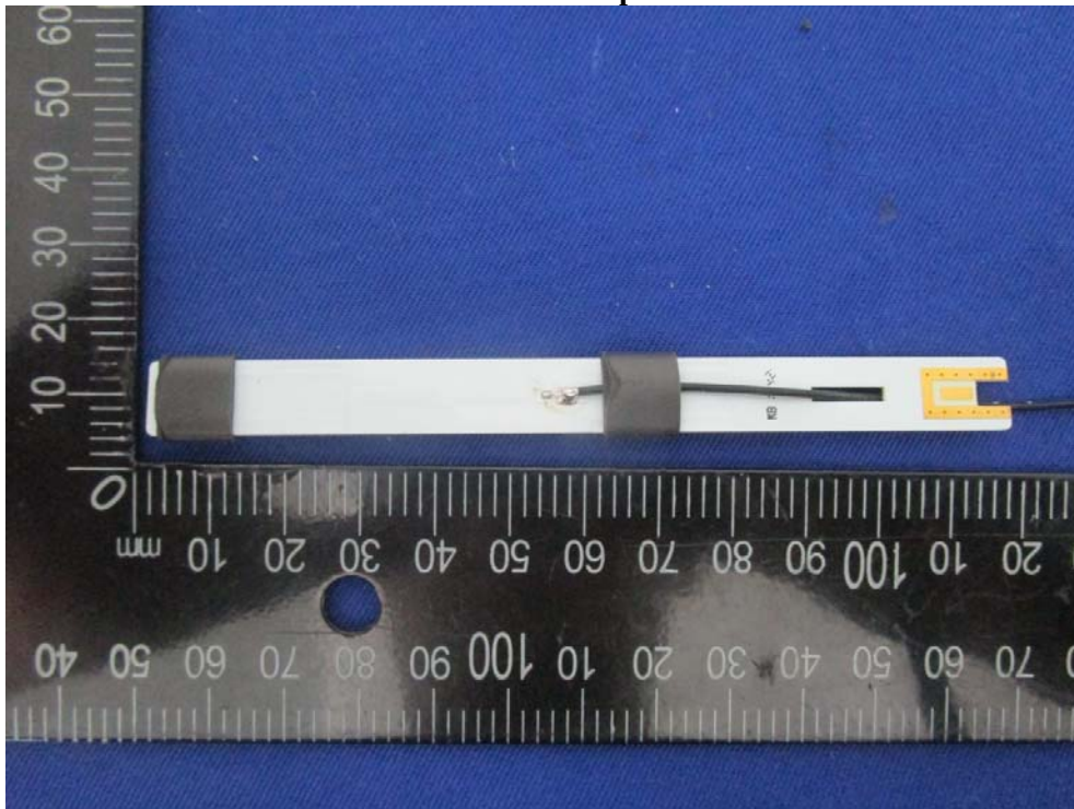
EUT – Ant Pcb Top View
