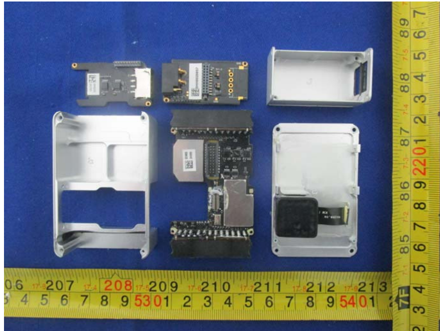
EUT – Flight Control Module Uncover View
