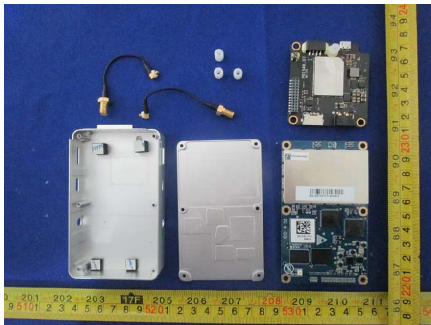
EUT – RTK Module Uncover View
