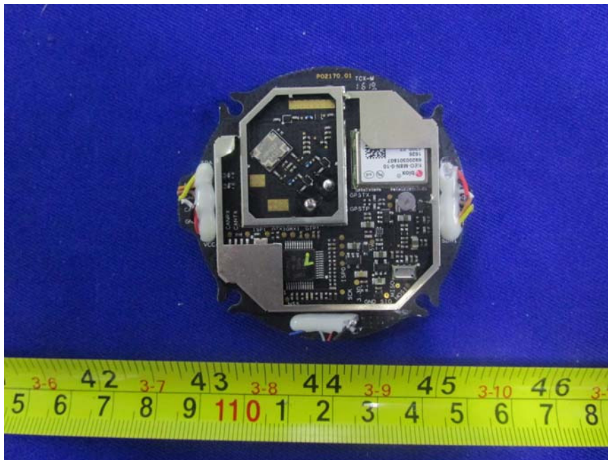
EUT- GPS Module-2 Top Unshielded View
