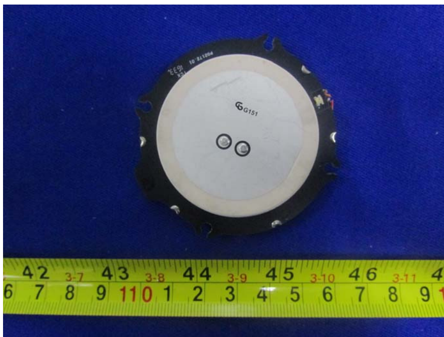
EUT-GPS Module-2 Bottom and Antenna View
